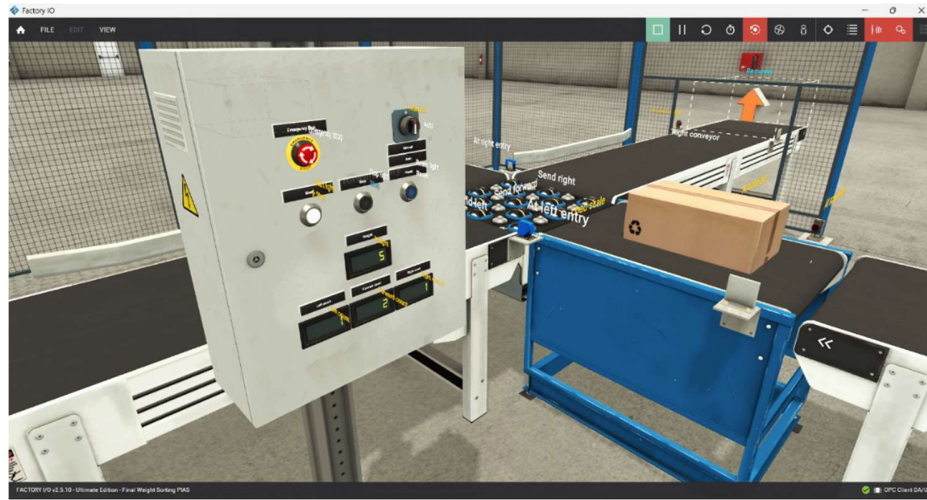
Fig. 4.4 Weight measuring sensor (load cell) configuration in Factory IO.
